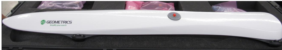
Figure 1 Using the internal GPS patch antenna by removing the external helical antenna.
