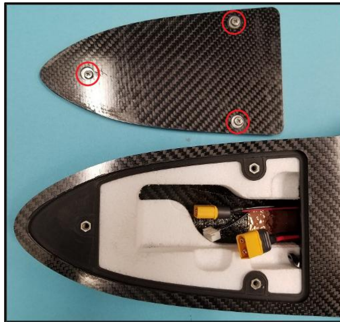
Battery Compartment Door Removed
