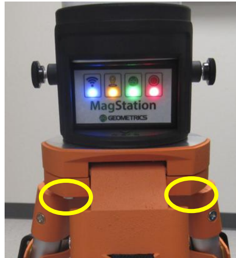
Figure 4-1 – Facing north or south guarantees the sensor will work anywhere in the world. Lock down the set screws to prevent tripod legs from splaying out.
