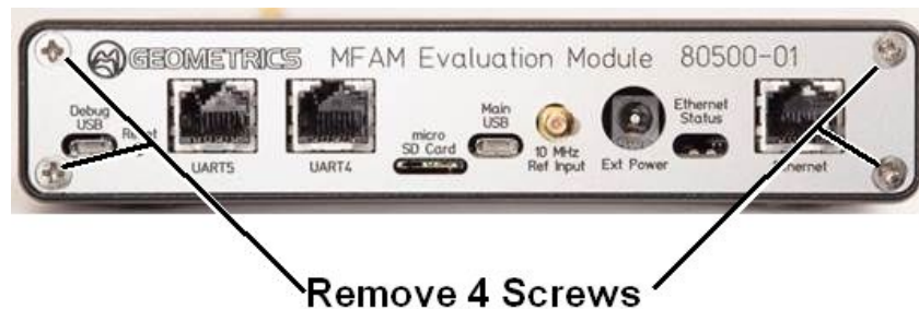
Figure 2 Showing 4 screws/ Removing Lid Specifications
