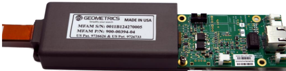
Figure 1: Ethernet Adapter Board with MFAM Sensor Module
