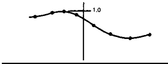
Figure 23. Aspect Factor (Relative Intensity of Dipole of Figure 21 with Respect to Angle from Axis at Various Points Along Profile)
