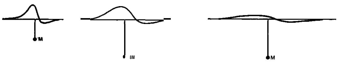
Figure 44. Depth/Amplitude Behavior of Dipole Anomalies
