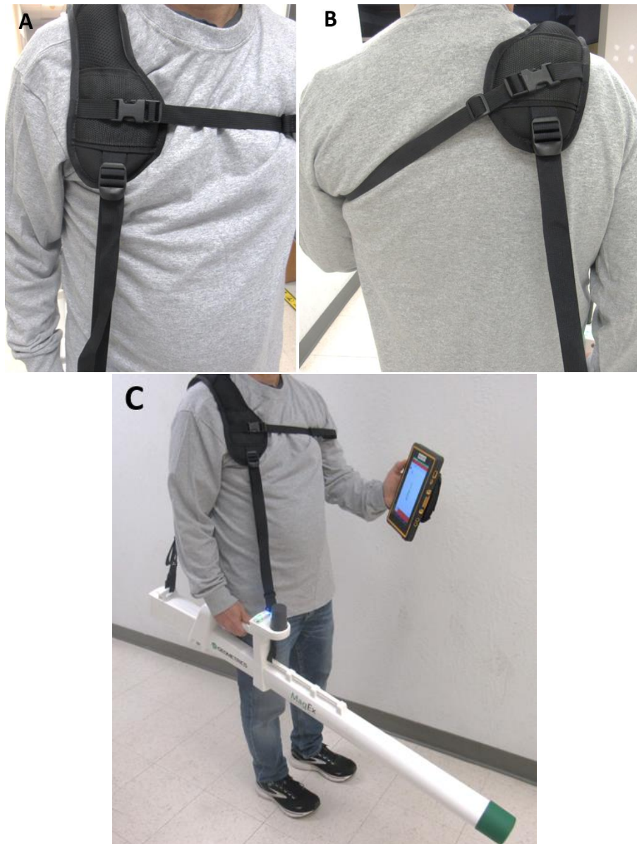
Figure 6-1 – Fitting the Shoulder Strap (A) Front View (B) Back View and (C) View showing the correct adjustment of the leveling strap.
