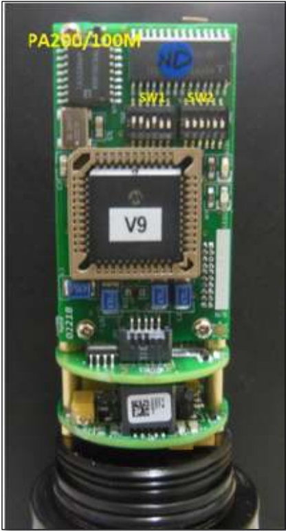
PA200: Switch 2 configured for 100M.
