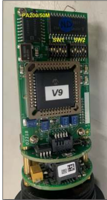
PA200: Switch 2 configured for 50M
