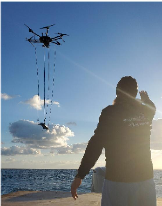
Figure 1 – Photo from a UAV magnetic survey performed over the shallow waters off the coast of Florida.
