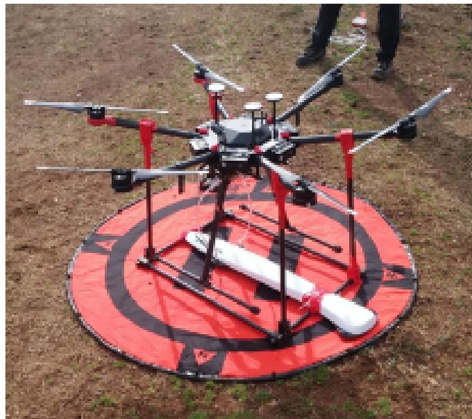
Figure 2 – Geometrics MagArrow Magnetometer affixed to a DJI M600 UAV with a rigid frame.
