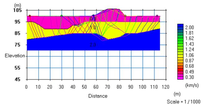
Set-up shots and receivers and perform a simulated survey. Adjust shot and receiver spacing to optimize coverage and minimize field time.
