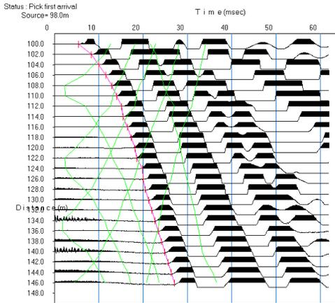
Go to the field and collect your data. Pick breaks quickly and accurately with the automated picker and adjust them manually with an interactive cursor. View travel times from other shots simultaneously for best coherence.
