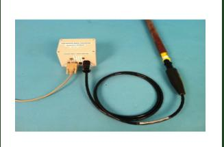
Data logging box connected to serial cable Can also be used with a Bluetooth Adaptor to connect to an Android phone or tablet.
