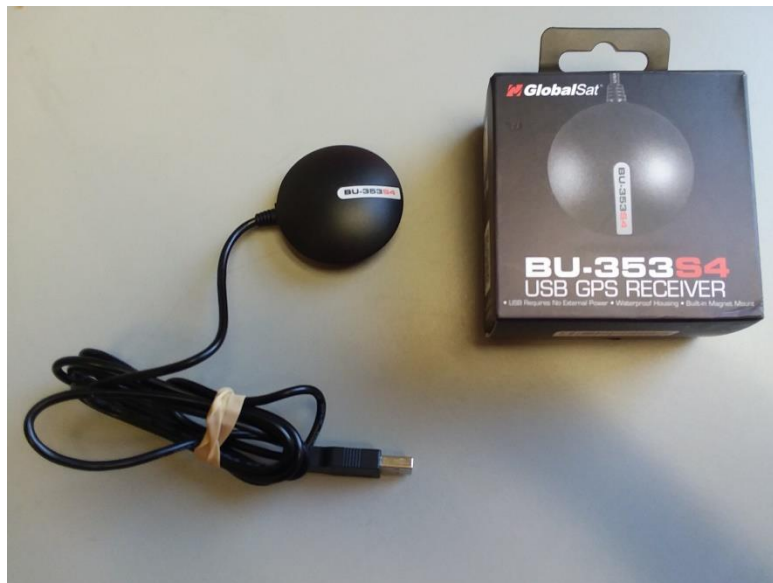
Fig. 7 GPS receiver with USB cable and GPS antenna (black)
