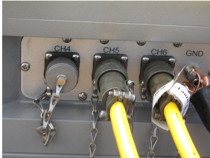
Fig. 13: Hy and Hx connected disabling E channels 6 and 5 respectively
