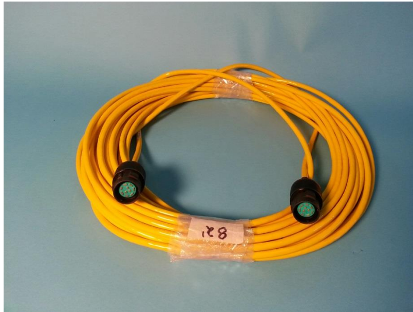
Fig. 6: Ethernet cable with 10-pin connectors on each end.
