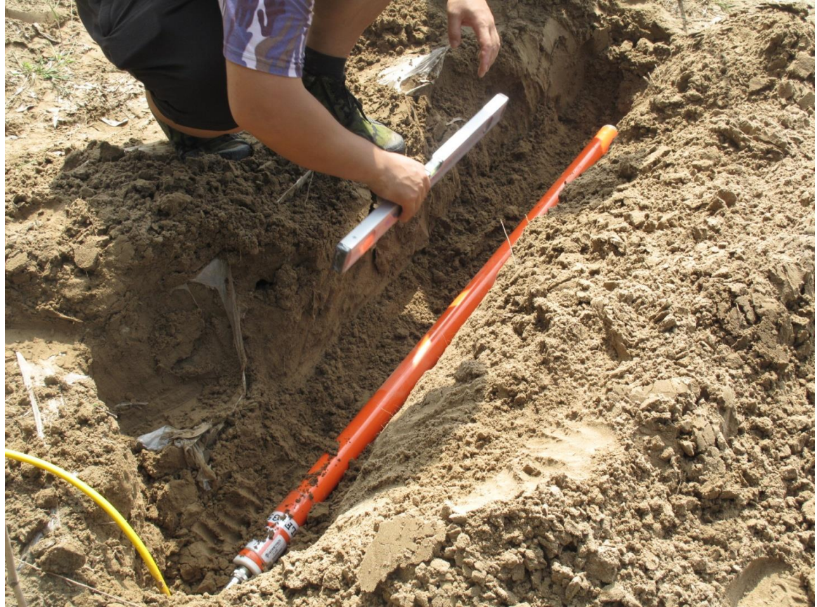
Fig. 17: Burying G20K magnetic coil
