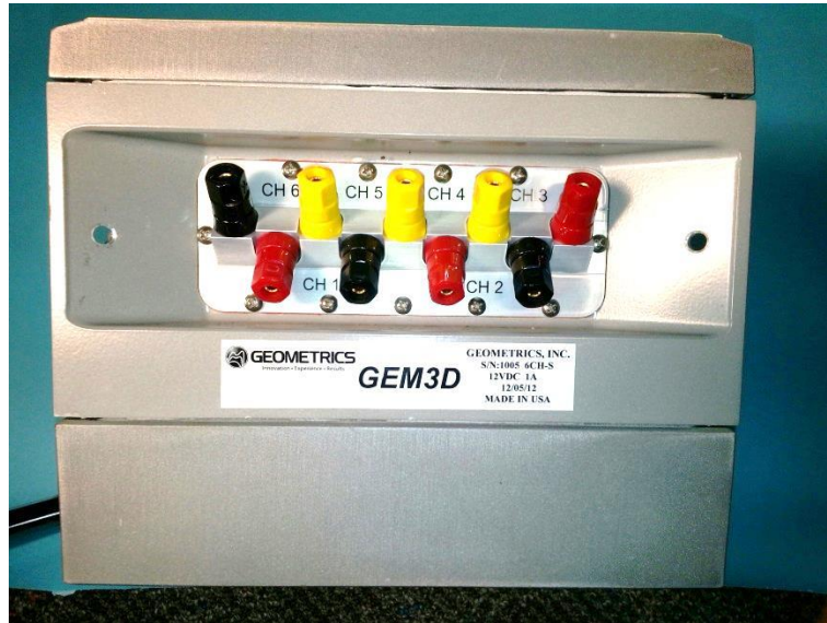
Fig 10: GEM3D receiver E-field (telluric) connectors
