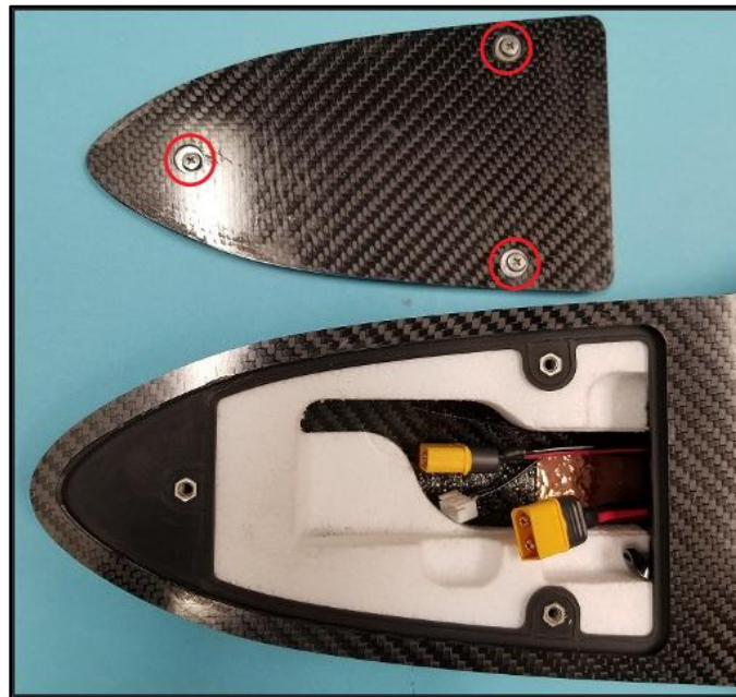
Battery Compartment Door Removed
