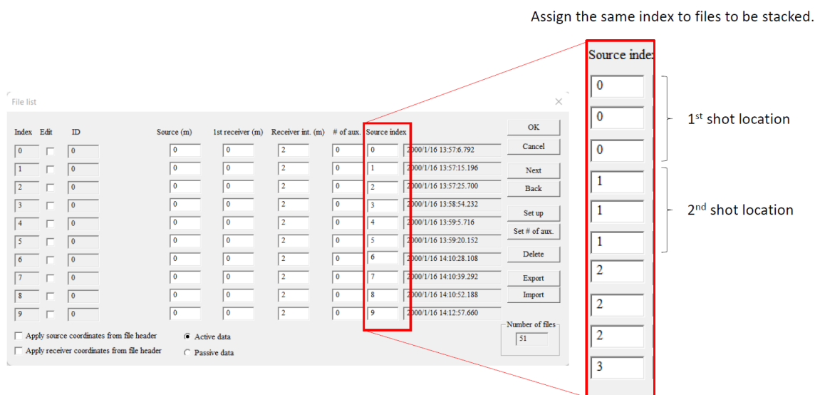
Figure 116: Setting up source indices prior to vertical stacking.
