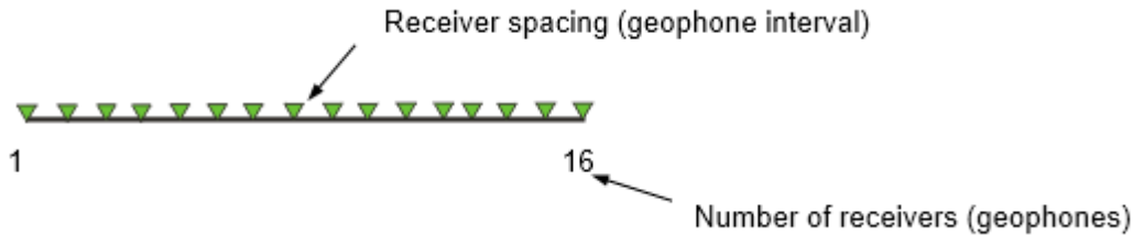
Figure 10: MAM survey linear spread configuration using all channels, one per geophone.
