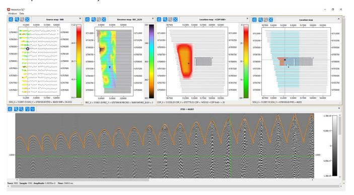
Geometry control by first-breaks – off-line and in the real time
