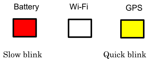
Figure 7.3 LEDs when data is being recorded with a very low battery
