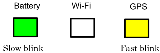
Figure 7.1 LEDs while data is being recorded (full battery).
