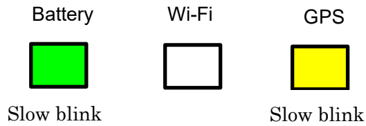
Figure 6.4 LEDs when Atom is locked on the GPS.
