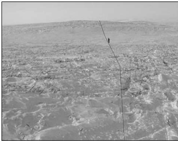
Figure 7. Transect of the resistivity and GPR surveys at Site 208. The surveyor is facing north and standing in the center of what appears to be a thaw depression.
