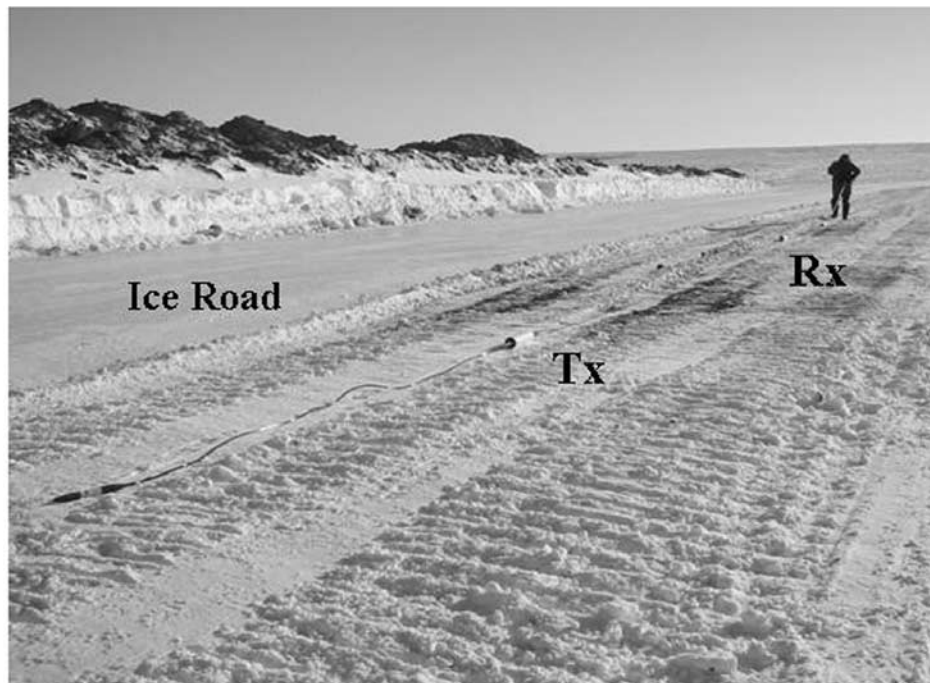
Figure 3. CCR data being collected along survey line at the outwash site. The left side is west, and the right side is east. The transmitter (Tx) and receiver (Rx) are shown. The sump in Figure 2 is located 4 m to the left (north) of ice road.
