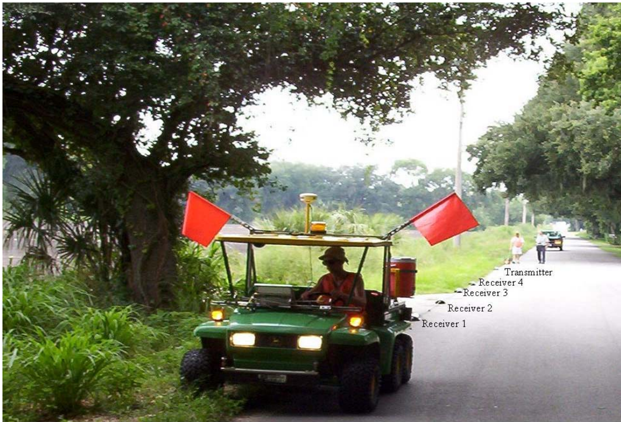
Figure 2.: Survey along a roadway using a four-channel Ohm-Mapper.
