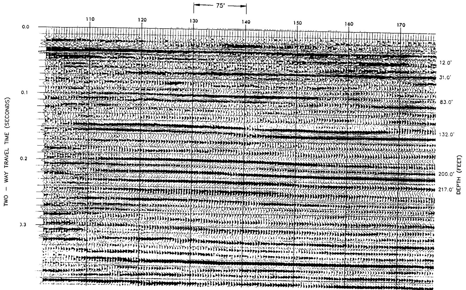
Figure 6 -Portion of S-wave reflection profile obtained from the final field experiment at Cooke Crossroads Test Site
