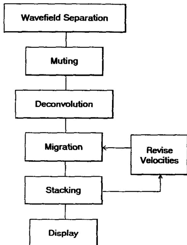
Fig. 4. Outline processing sequence for crosshole seismic reflection data.
