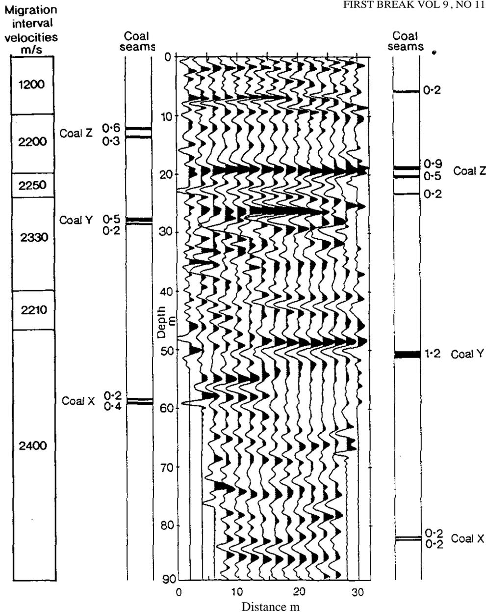
Fig. 6. Final section with prestack depth migration from a survey across a normal fault zone. The velocity field used for migration is displayed to the side.
