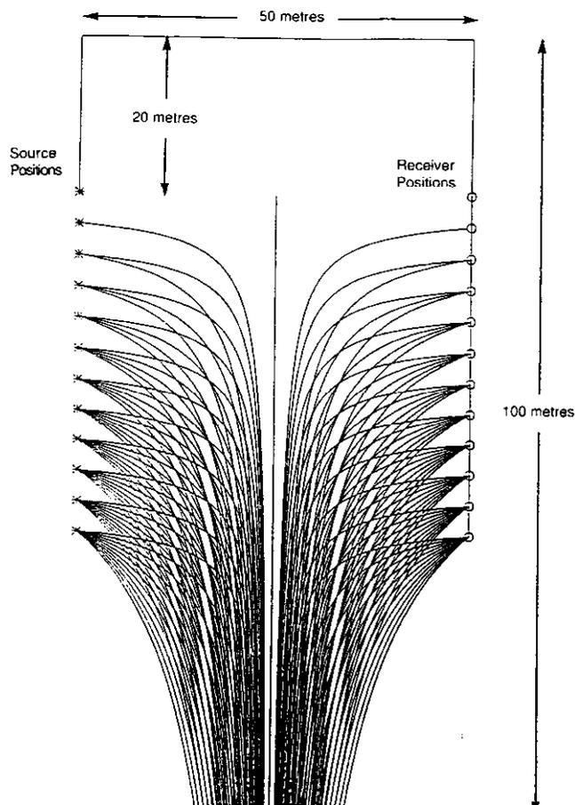
**Fig. 3. Reflection point loci** for upgoing primary reflections in a crosshole survey of typical dimensions. Only alternate source and receiver positions, at 4 m spacing, are shown for clarity.
