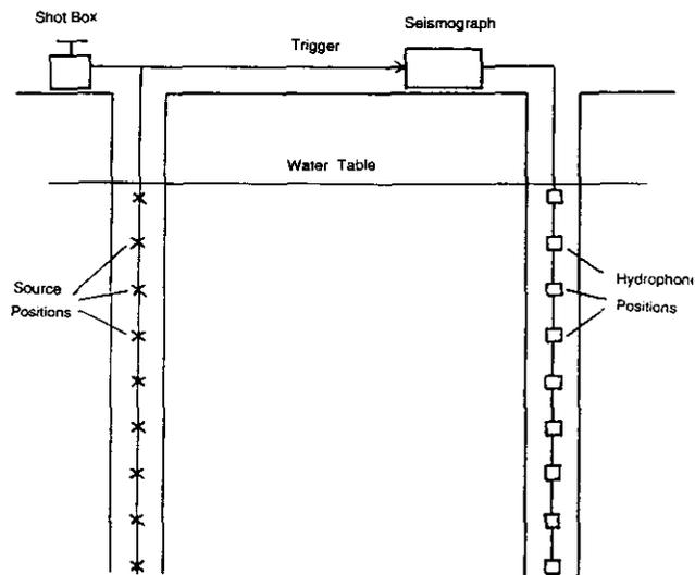
Fig. 1. Schematic diagram of field set-up for data acquisition. Borehole separations are typically 30–60 m and source and receiver spacings are 2 m over a depth range of 40 m or more.
