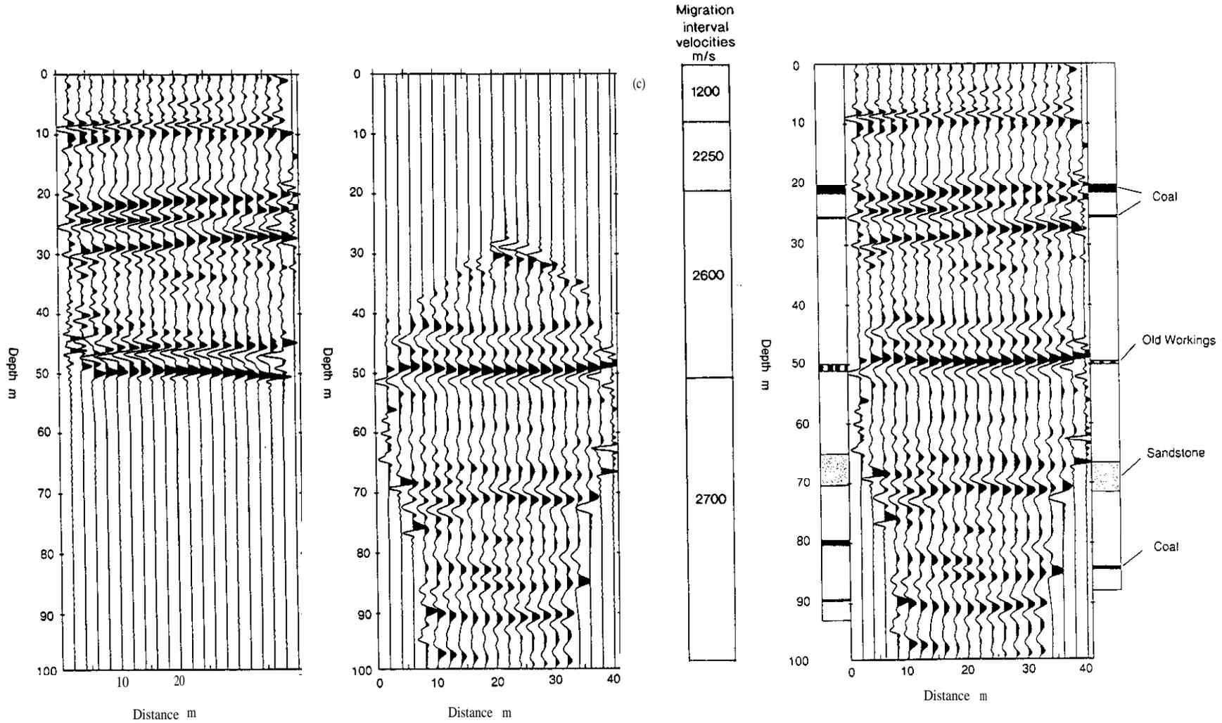
Fig. 5. Stacked sections with prestack depth migration from an example survey: (a) downgoing wavefield; (b) upgoing wavefield; (c) combined up- and downgoing wavefields. The velocity field used for migration is displayed to the side.
