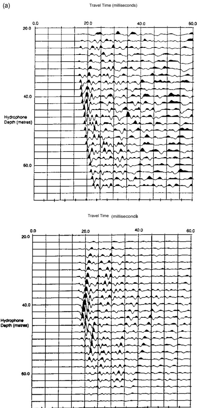
**Fig. 2. Common-shot** gather from a detonator at 30 m depth with hydrophones over the depth range 22–66 m: (a) raw data with gain ramp applied proportional to travelt ime squared; (b) showing only the upgoing wavefield at the receivers after wavefield separation in the  $f$ - $k$  domain.
