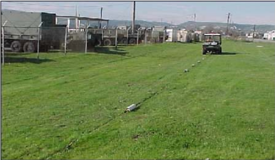
Figure 2. Photo of the OhmMapper during operation at Camp Parks. The mule is in the foreground pulling the OM array.
