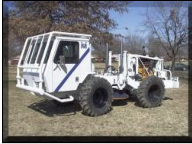
Figure 2. Buggy-mounted vibrator (courtesy Industrial Vehicles International).
