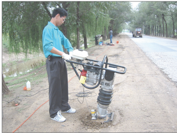
Inexpensive construction tampers are used for the energy source.
