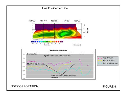
Typical results of the Geometric's OhmMapper investigation are show on colored resistivity cross sections on Figure 4 for the lines shown on Figure 2. A comparison of inverted Geometric's OhmMapper results and test pit drag line results (Figure 4) indicate a reasonable correlation of the low resistivity areas and locations that peat/muck was excavated.
