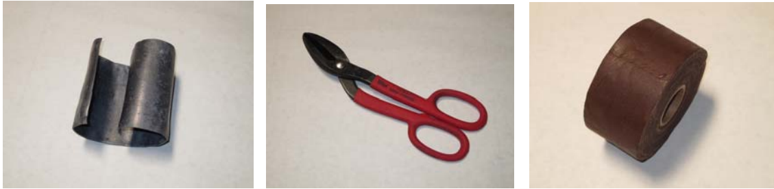
Figure 9. Sheet lead, tin snips, and Bulldog tape.
