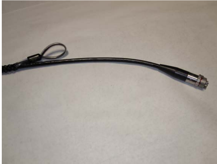
Figure 5. Tow cable 55-pin connector termination shown with Kellems grip.
