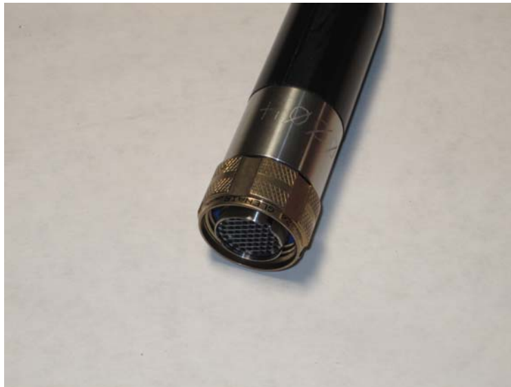
Figure 4. Deck cable 55-socket connector termination.
