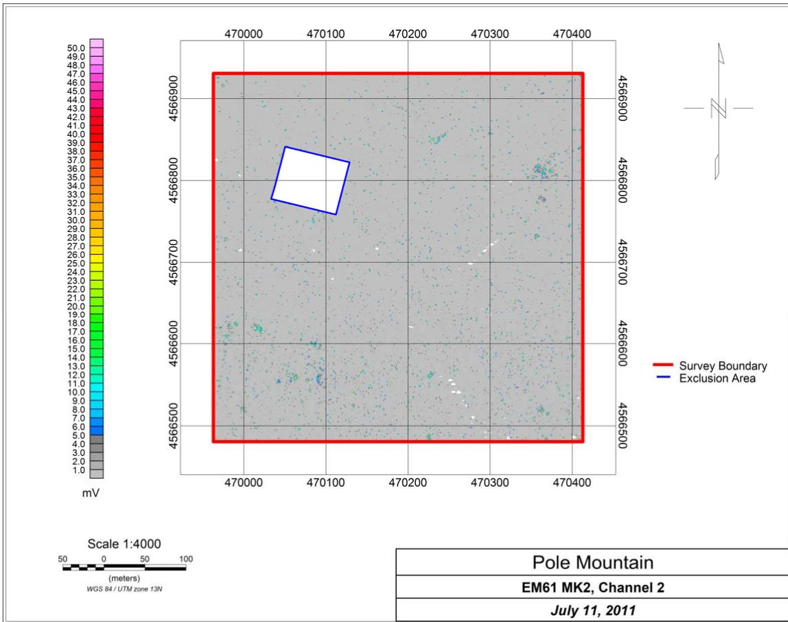
**Figure 5. PMTMA EM61-MK2 Production Data Channel 2 Survey Results**
