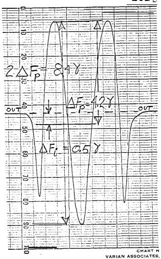
Figure 1. Rotation of rifle in a vertical N-S plane at the end of a horizontal E-W line of known length. The perturbation on the total field from the effects of the permanent moment is noted as AF present moment moment effects either increase or decrease the total intensity whereas the perturbation  $\Delta F_{i}$ , from the induced moment always adds to the total intensity when the Long dimensions of the object are parallel to the field.
