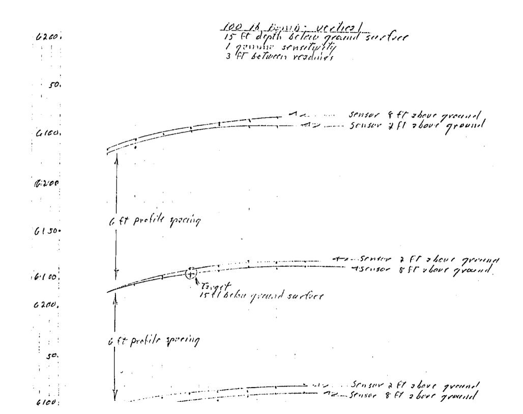
100 16 bomb - vertical 15 ft depth below ground-surface 0.25 gamma scinstituity 3 ft between readings ----- sensor aft above ground Target 15 ft below surface
