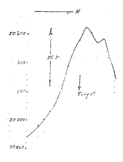
250 16 bomb - Vertical 9 Ft depth Deless ground surt: sensor 8 ft above ground 025 junme sensitivity
