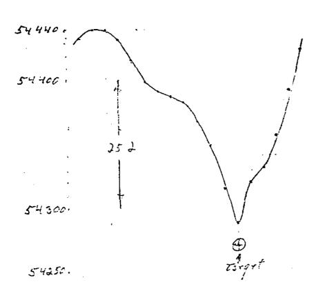
750 16 bemb-vertical 18 ft depth belens surta sensor 2 ft above surface 14 gamma sensitivity 2 ft between readings
