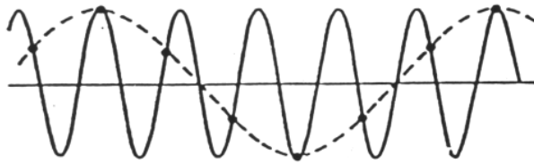
Figure 8. Example of spatial aliasing (from: Anonymous, 1966). The solid line is the signal of interest. The spatial separation of samples (solid dots) is large compared to the wavelength of the signal (solid line), and the signal reconstructed from the samples (dashed line) has a different wavelength than the signal of interest. This highlights the need for the spacing of discrete measurements to be small in comparison to the expected wavelength(s) of the signal that one seeks to observe.
