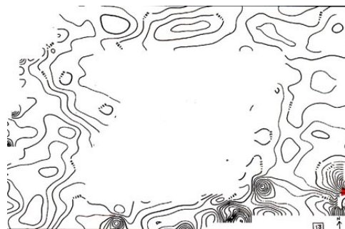
Figure 7. Contour map of magnetic intensity over Monument 61 (shown in Figure 6). The head was found under the anomalous area indicated by the colored marker in the lower right-hand corner of the map. The area at the center of the map was covered by a large artificial pond, where no measurements were made.
