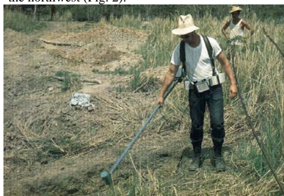
Figure 3. Surveying the San Lorenzo site with the magnetometer.
