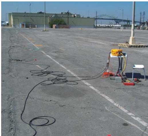
**Refraction Microtremor Array Layout**
