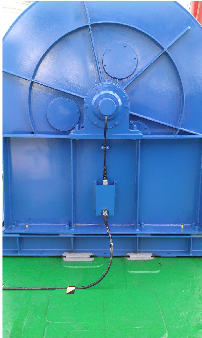
*Figure 14: Right-angle Repeater installed on a winch between Deck Cable and Tow Cable.*
