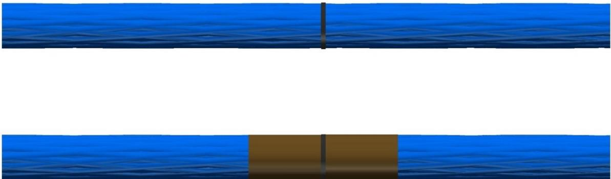
Figure 87: Rope markings for Interconnect Cable installation.
