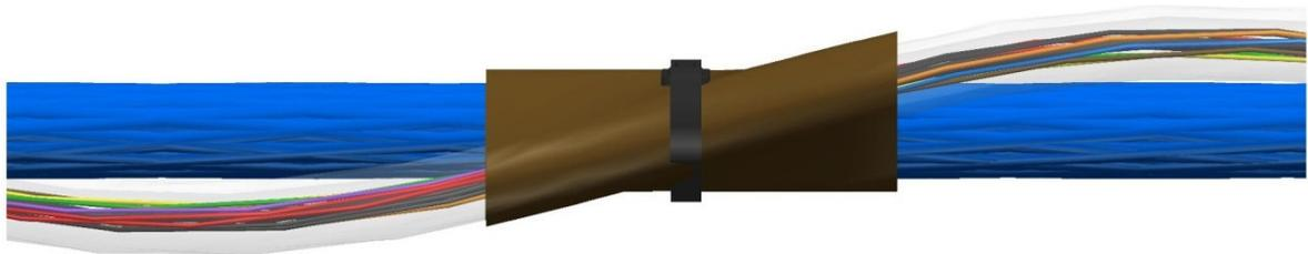
Figure A 91: Zip tie installed on Cross Cable.
