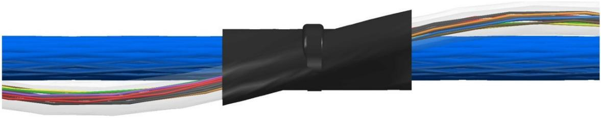
Figure 92: Plastic tape installed and secured with the " pull-through" method.
