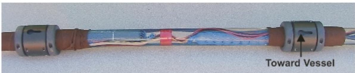
*Figure A122: Complete set of collars installed on streamer.*
