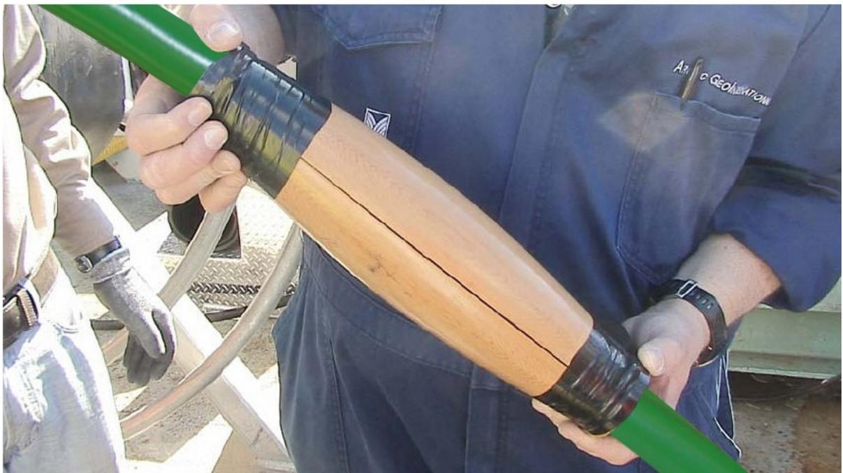
*Figure A125: Tape applied over tie wraps to protect Streamer.*
