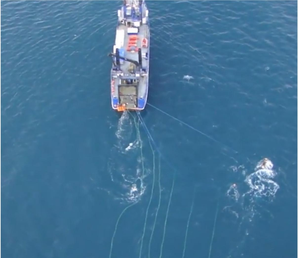
*Figure A144: Picture of array just prior to deployment of Port paravane.*
