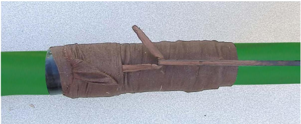
*Figure A135: Finish friction tape termination.*
