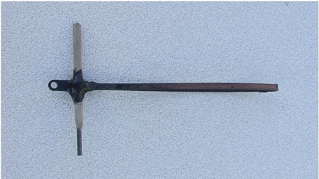
*Figure A131: Simple tool fashioned out of welding rod and tie wrap.*
