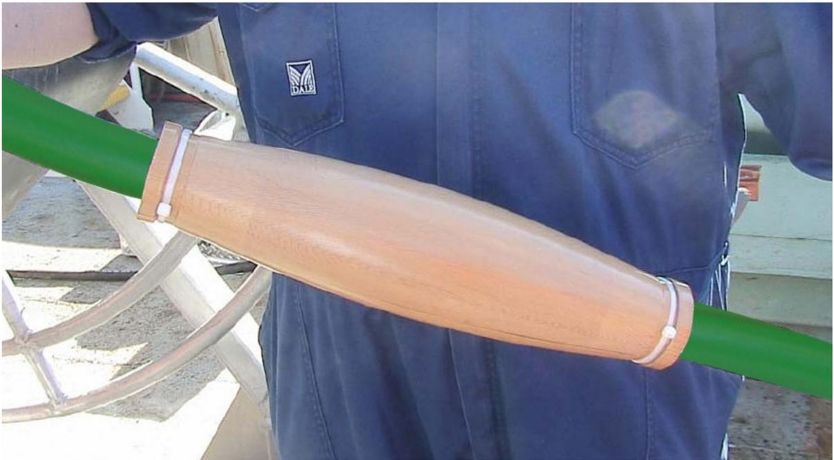
*Figure A124: Digitizer float secured to Streamer with tie wraps.*
