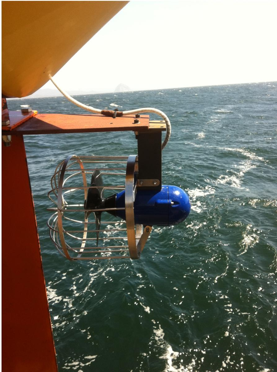
*Figure 42: Turbine mounted on paravane.*
