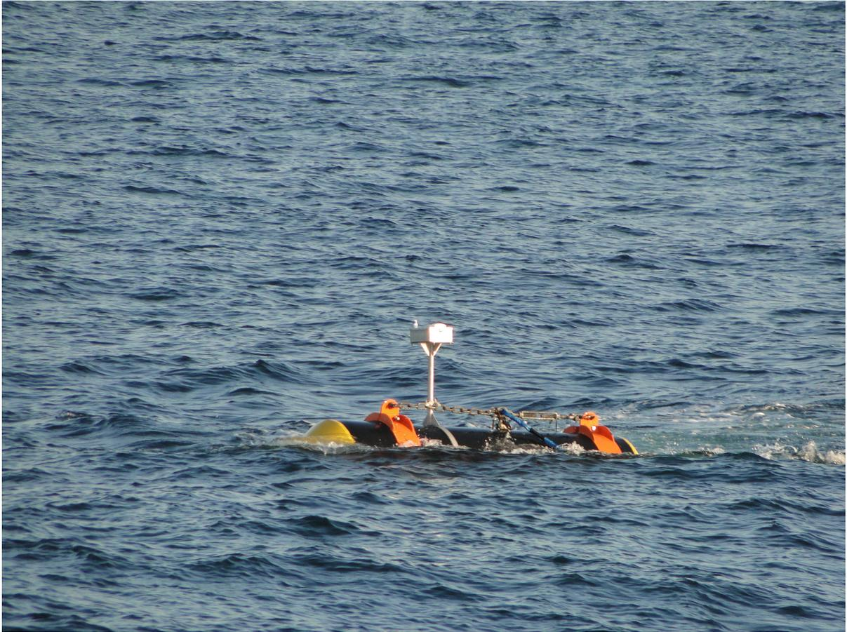
*Figure 43: Paravane-mounted GPS.*
