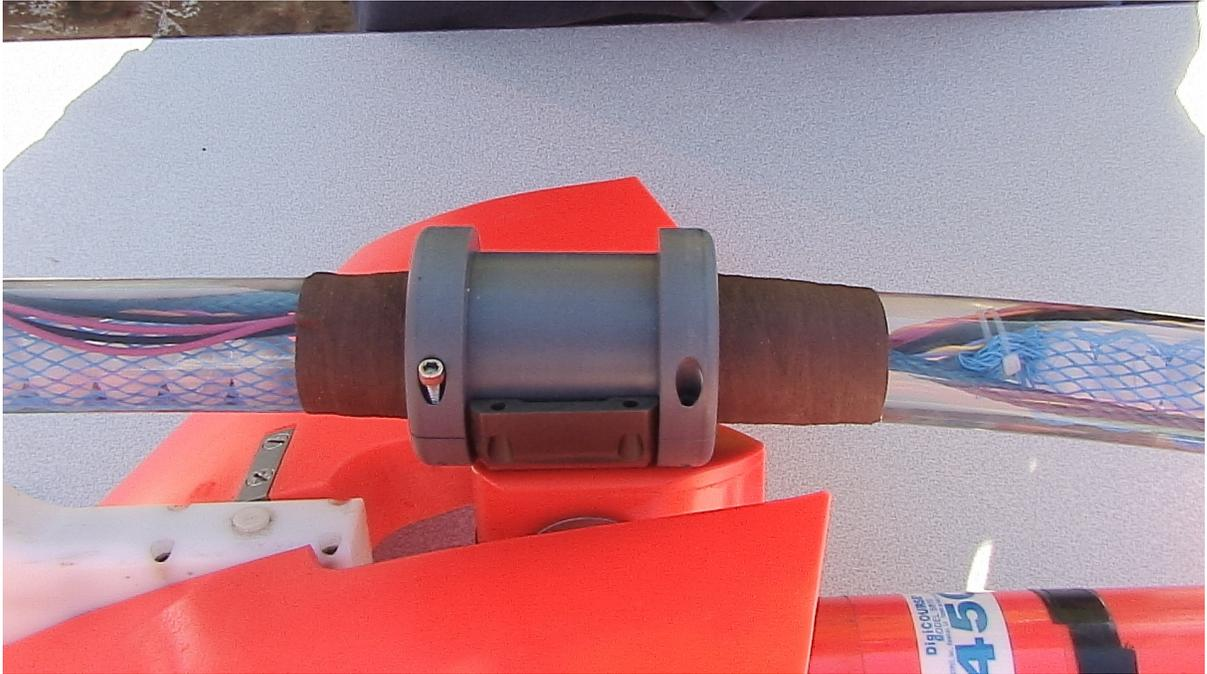
*Figure A120: Aligning installed inboard collar to assist alignment of outboard collars.*
