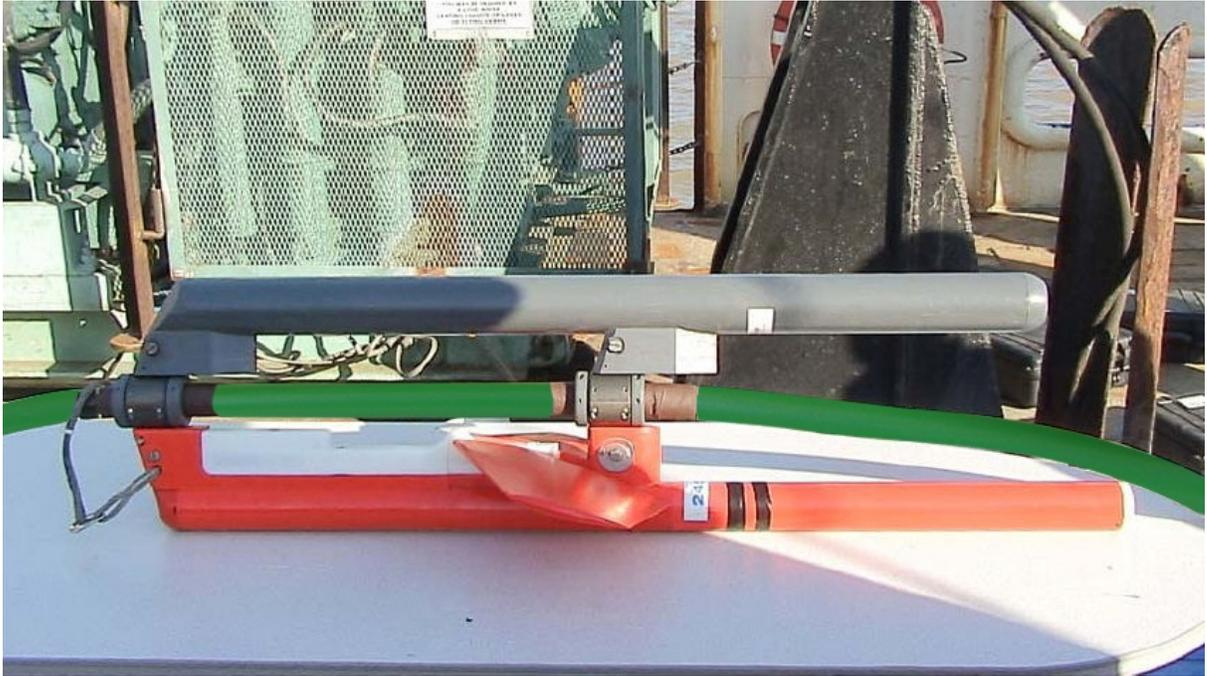
Figure A123: Complete bird and bird float installation.
