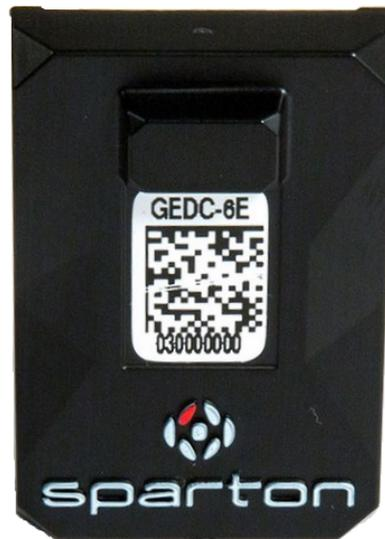
*Figure A157: Sparton GEDC-6 Digital Compass.*
