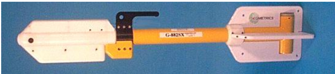
Figure 1 G-882 Tow Fish with nose mounted echo-sounder altimeter housing
