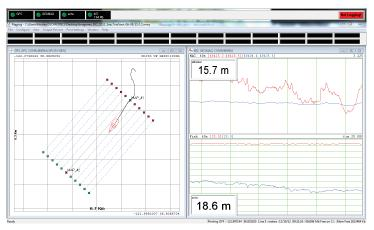
MagLogLite<sup>™</sup> Data Logging software is included with each magnetometer and allows recording and display of data and position with automatic anomaly detection. Additional software options include: MagLog Pro<sup>™</sup>, advanced logging software; MagMap<sup>™</sup>, a plotting and contouring package; and MagPick<sup>™</sup> post-acquisition processing software.
