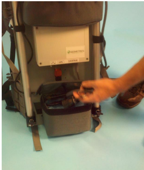
Figure 10B Locating power cable connector, mount connector on junction box power plug
