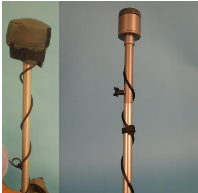
Figure 9A & 9B Showing GPS cable routing Left: NovAtel GPS Right: Tallysman GPS
