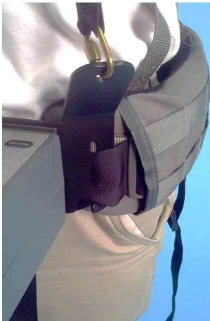
Figure 25 Thread black console belt through tangs on “attachment bar” on console
