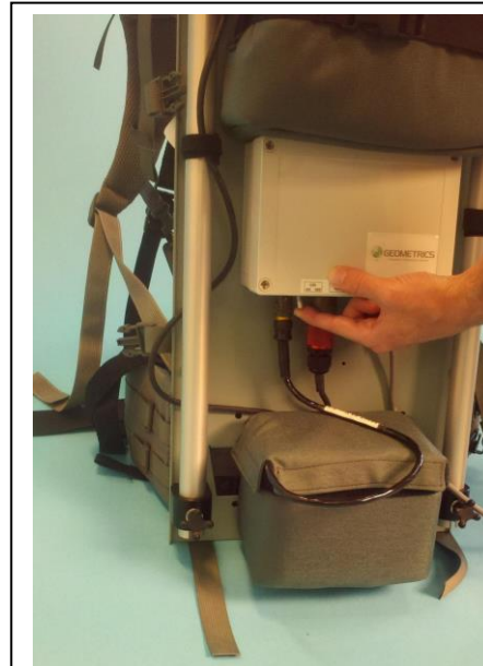
Figure 11 Showing GPS Power Switch
