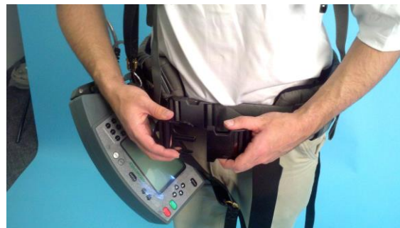
Figure 24B Secure secondary console belt
