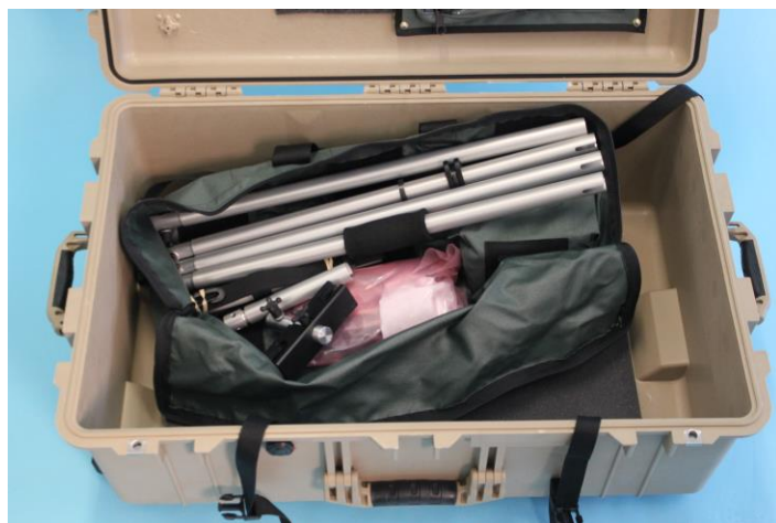
Figure 7 Case and bag with GPS and sensor staff sections
