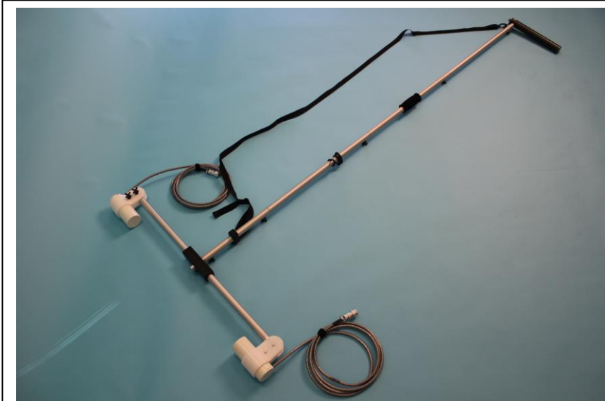
Figure 18 Complete assembly of staff with sensors
