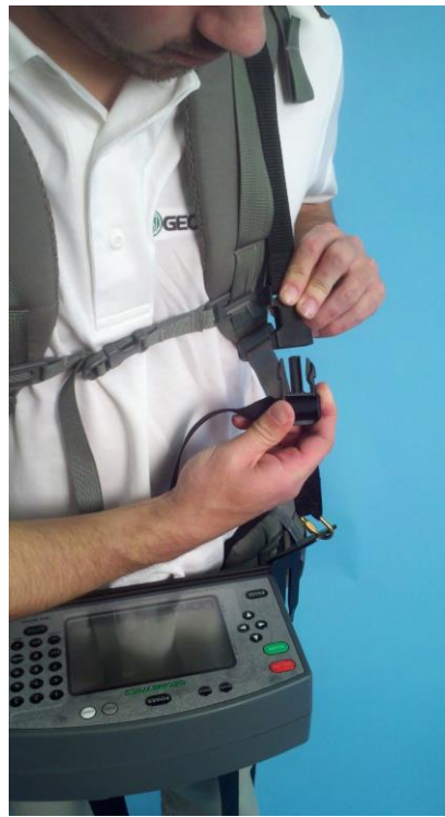
Figure 26A Attach secondary lapel strap for console support
