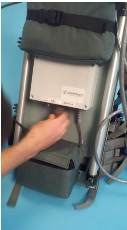
Figure 10A Attach GPS Cable to Junction box
