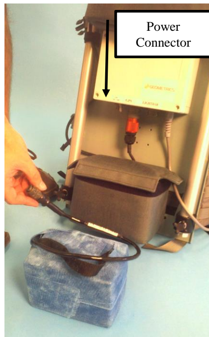
Figure 14 Locate Battery Connector
