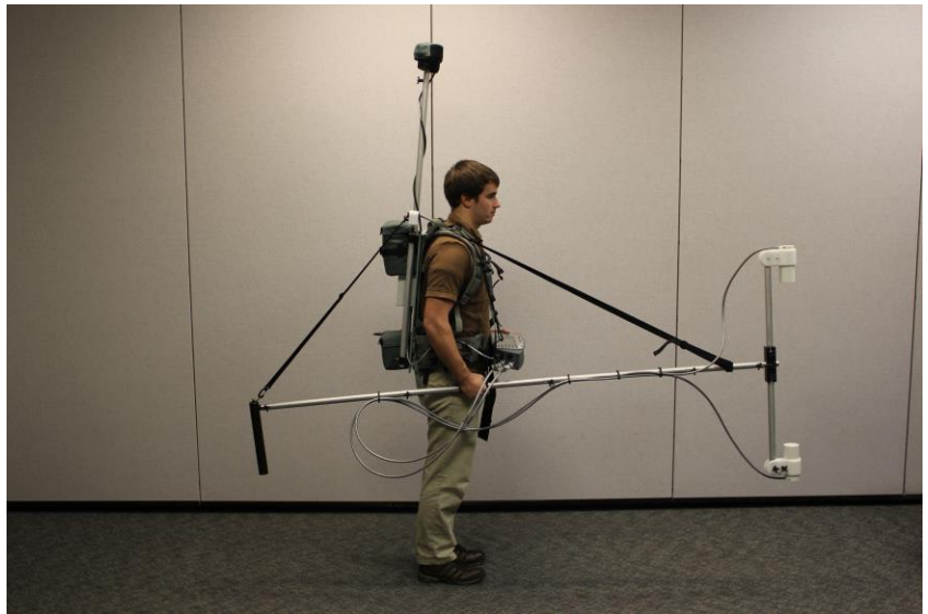
Figure 2 G-858GAP with forward staff deployment mode
