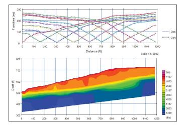
SeisImager/2D Lite refraction data analysis software lets you model and plan your survey beforehand. Pick first breaks and output cross-sections by two different analysis methods.
