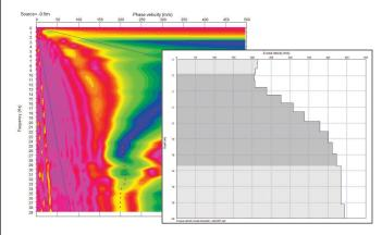
SeisImager/SW surface wave data analysis software calculates dispersion curves from active and passive source (microtremor) data records. The dispersion curves are then used to determine V<sub>5</sub>.
