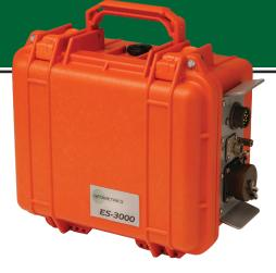
If you need a basic exploration seismograph for teaching purposes or to solve simple engineering problems, the ES-3000 is for you. The system includes the ESOS data acquisition software, and the ES-3000 seismodule connects directly to your PC via the Ethernet port – no additional hardware or drivers are required.
