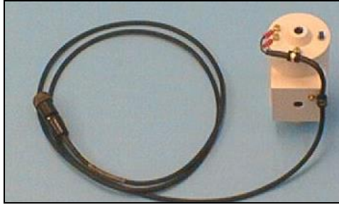
Figure 11. Top sensor with gradiometer cable attached
