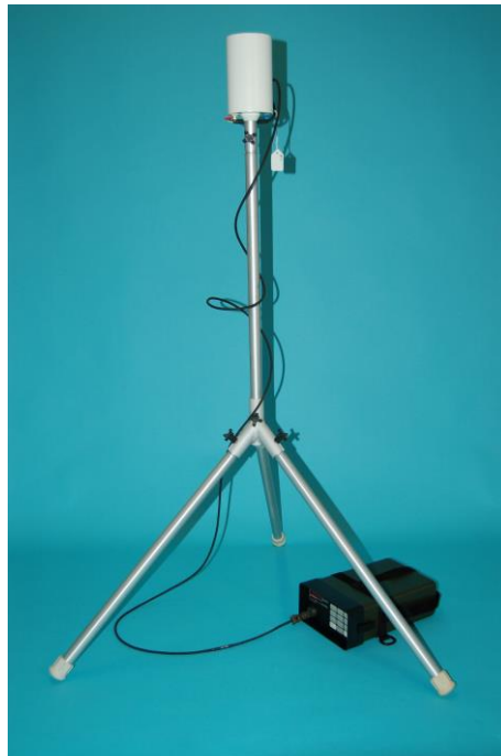
Figure 16. Base-station setup up using tripod kit and G-857 staff section
