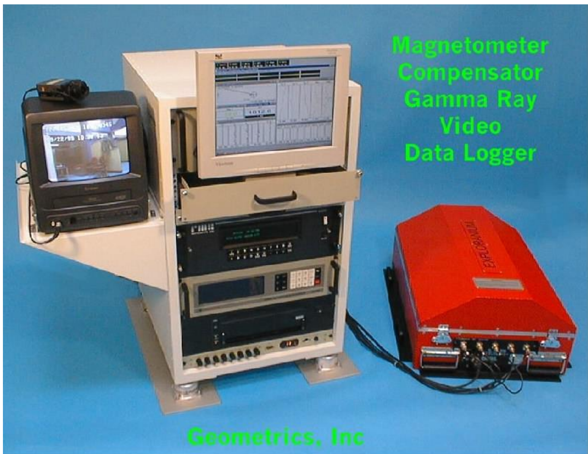
Figure A8. Rack mount for airborne geophysical survey system
