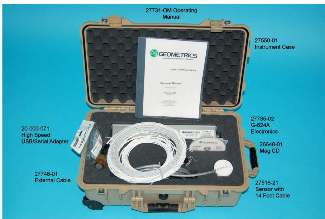
Figure 2 G-824 System and Accessories
