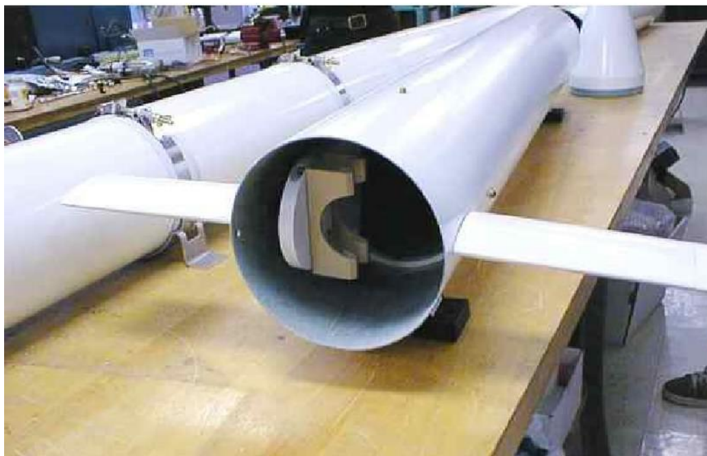
Figure A2. Airborne Stinger showing sensor mount.
