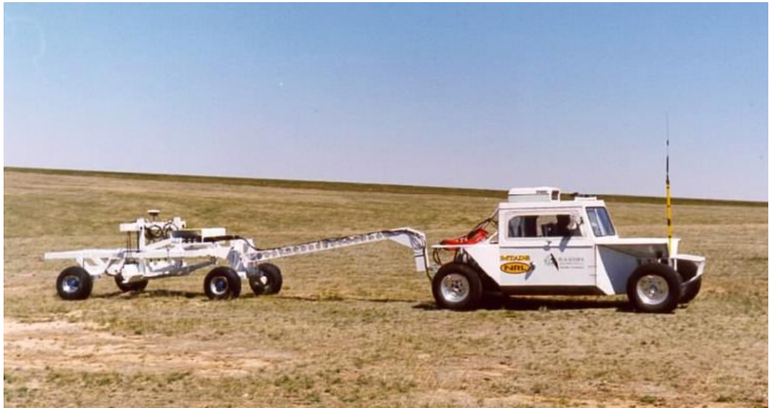
Figure A9. MTADS multi-sensor array for UXO survey applications.
