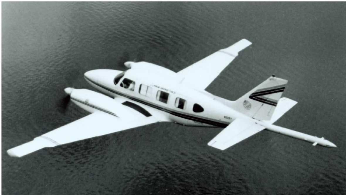
Figure A4. Aircraft fitted with horizontal transverse and longitudinal gradiometer using faired wingtips and stinger.
