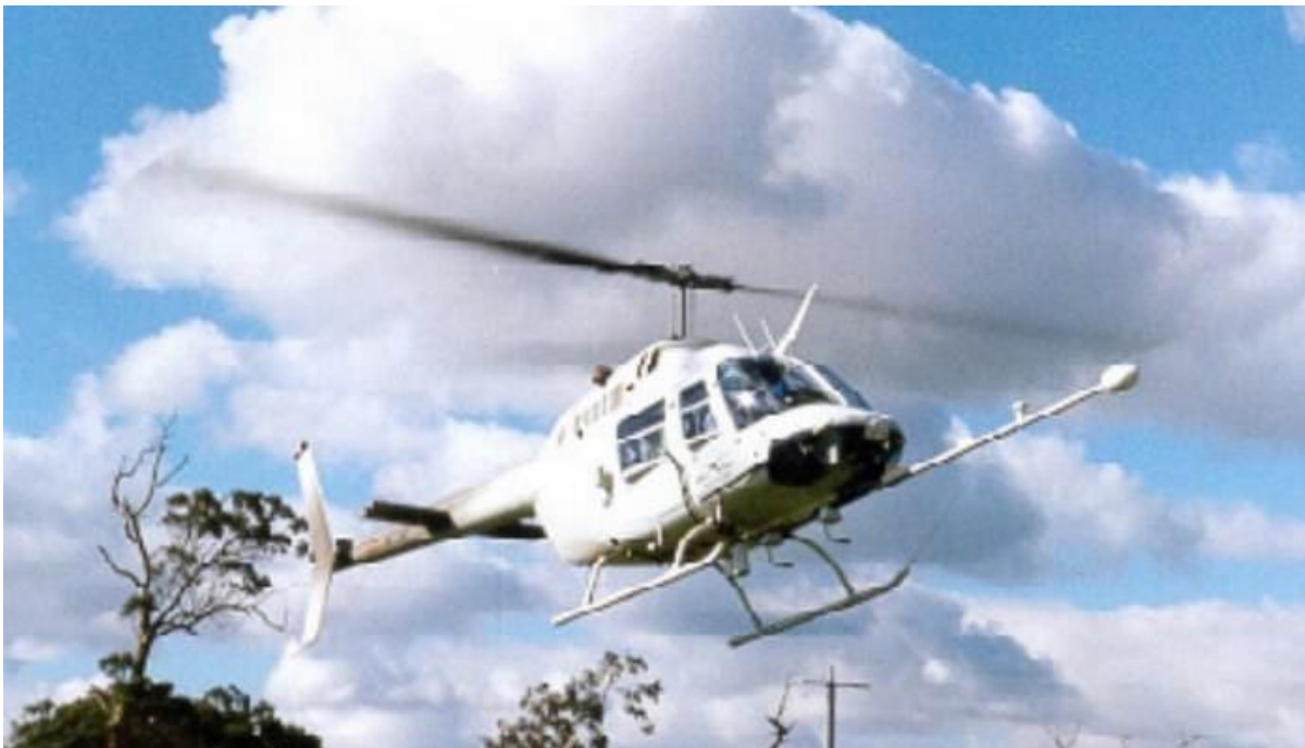
Figure A6. Single sensor boom installation on Helicopter.
