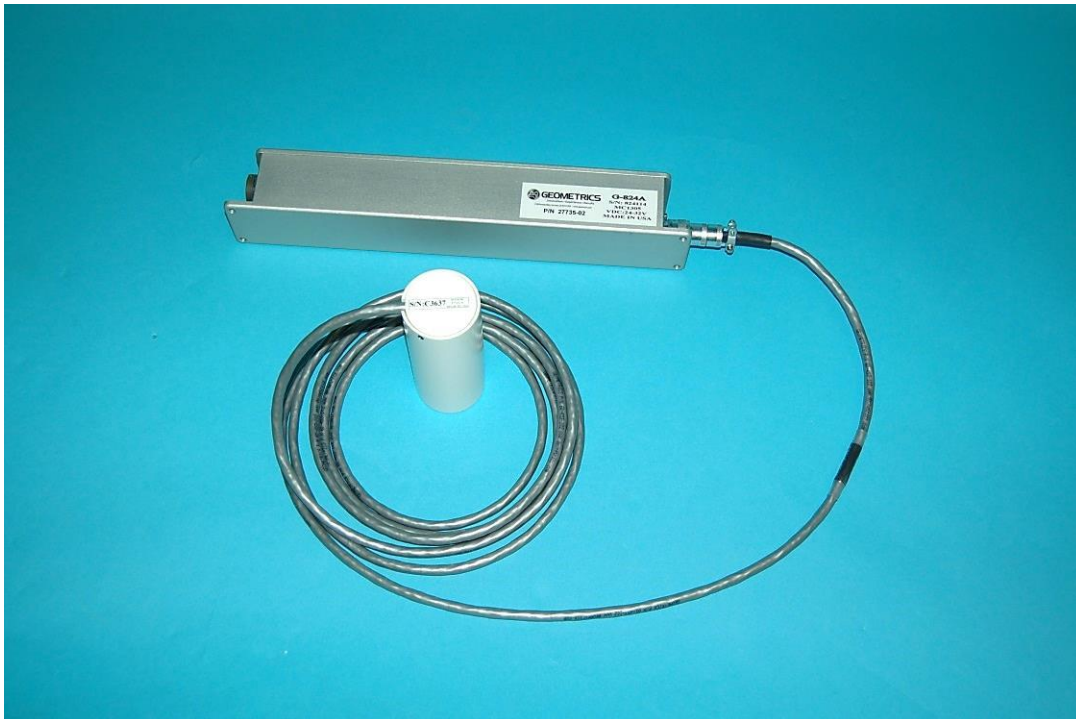
Figure 1 Sensor, sensor cable and Sensor Driver Module
