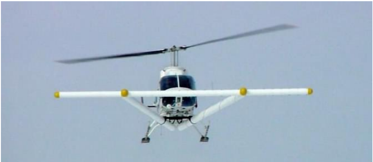
Figure A7. Multi-sensor (7) MTADS Helicopter installation for UXO survey.
