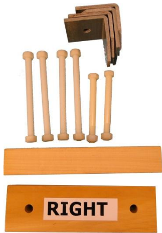
Figure 6 - Parts for attached Y-Transmitter Coil (Thicker Wooden Blocks)
