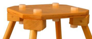
B) Top of GPS Platform
