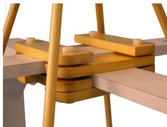
Figure 7 - Vertical transmitter coil stabilization blocks
