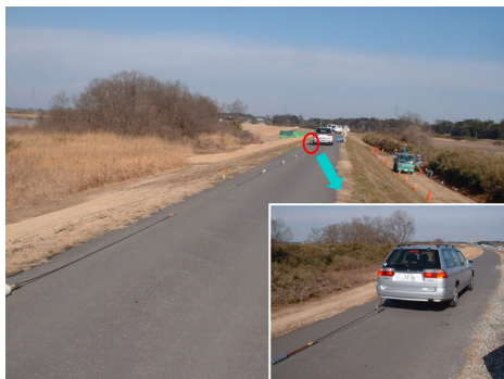
Figure 8. Photo of site(3); The OhmMapper in operation on the levee of the Kokai river.
