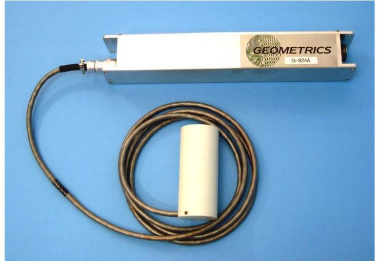
The Geometrics Model G-824A mates the well-proven high-performance cesium sensor with new sensitive internal sensor driver and Larmor counter electronics. Improved low noise amplifiers have now lowered the noise floor to approximately 300 fT (femto-Telsa). This advanced integrated magnetometer provides unmatched versatility in performance, small size, low weight, wide application range and cost effectiveness.
